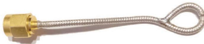
**Fig. 5.** Shielded magnetic field probe, before wrapping in an insulator to allow safe probing of any area of the device under test.
